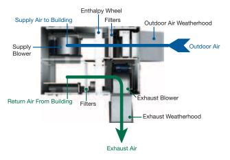
Utilizing an enthalpy wheel to precondition the outdoor air, narrows the operational range of outdoor air conditions which the building's HVAC equipment is designed to temper. It is this reduction in the outdoor air range that allows for size reduction in heating and cooling equipment and reduced energy costs.
